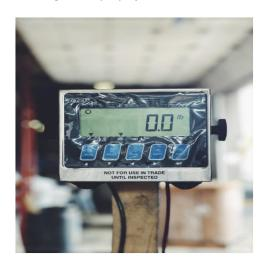
**Figure 2**The type of industrial pallet scale used for measuring the PLTs
