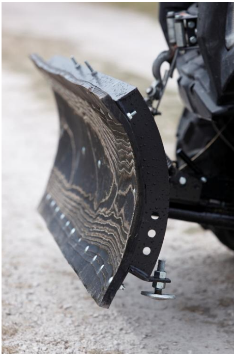
Innovative uses for Manitoba scrap tires helps to manage the 1.4 million scrap tires generated every year in Manitoba. At left: OTR Recycling of Ashern fabricates an OTR tire into an ATV Snow Plow Blade.
